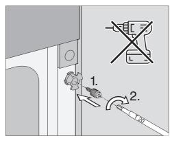
Insert the bolt into the mounting aid and tighten it in the cabinet niche. Do not use a cordless screwdriver.
