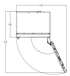
Max clearance required for opened door is 49-3/4" when opened to 90°\* (dimensions shown are without door overlay installed.)
