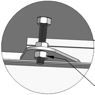
7.2 Tighten firmly the 4 nuts under the table.
