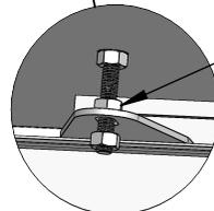
Screw or unscrew the 4 nuts on the plates.
