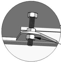
Unscrew the 4 nuts under the plates.
