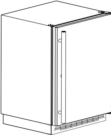
2. Place shell accessory over front and back of cabinet base, aligning holes of shell accessory with the holes on the base. Insert sheet metal screw in back of base.
