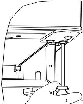
2. Remove corresponding screws on opposite side of cabinet. On some models there may be a nut behind one or both screws on either side.
