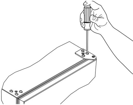
3. Remove door by tilting forward and lifting door off bottom hinge. Retain shoulder washers; they will be reused.
