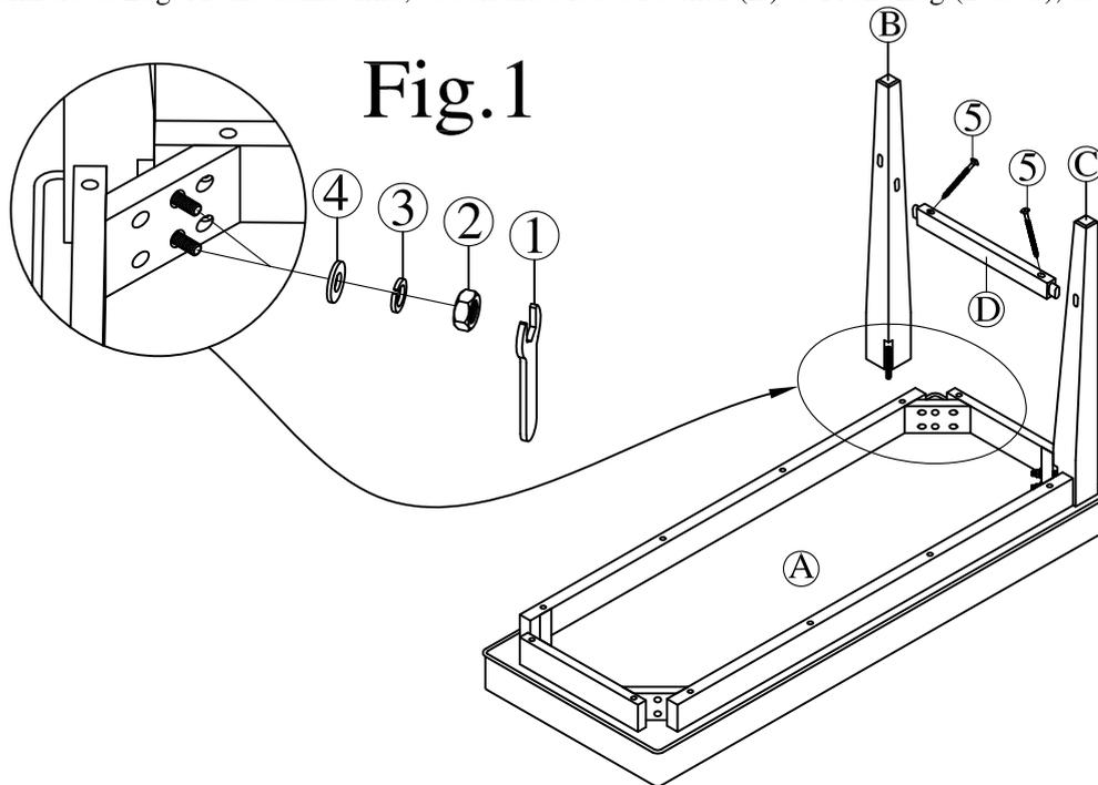
**Step 2:** Assemble Side Stretchers (D) to Front Leg (B & C) using Wood Screw (5). Attach the Front Stretcher (E) to the Front Leg (B & C), using Wood Screws (5). At the same time, attach the Front Leg (B & C) and Side Stretcher (D) to the Seat Frame corner (A) and secure with Flat Washer (4), Spring Washer (3) and Hex-Nut (2). Tighten Hex-Nut (2) with Wrench (1). Repeat this step for the remaining Front Leg, Front Stretcher and Side Stretcher.
