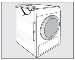
The tumble dryer must stand perfectly level to ensure safe and proper operation.
