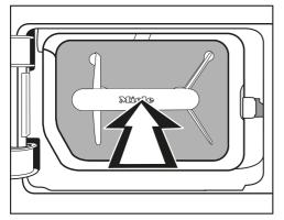
2 Then press on the handle until the lint filter is secured in position.
