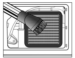
Carefully vacuum up any visible lint or soiling. Use a dusting brush or the narrow crevice nozzle.
