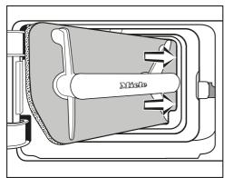
① Use the handle on the right to slide the lint filter at an angle behind the edge.
