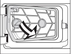
Use the handle to pull out the filter insert <u>at an angle</u> forward and to the right.
