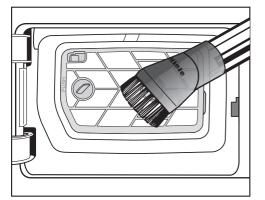
Carefully vacuum up any visible lint or soiling. Use a dusting brush or the narrow crevice nozzle.
