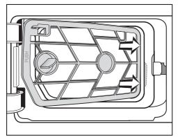
1 Use the handle on the right to slide the filter insert <u>at an angle</u> behind the edge.
