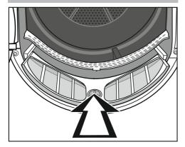
■ Push the lower lint filter in completely and lock it with the yellow knob.
