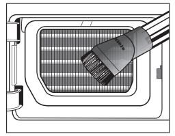
■ If you notice any visible soiling, carefully vacuum it up with a vacuum cleaner. Use a dusting brush or the narrow crevice nozzle.
