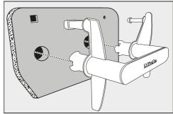
■ Place the lint filter back on the handle. Make sure it is the correct way round.
