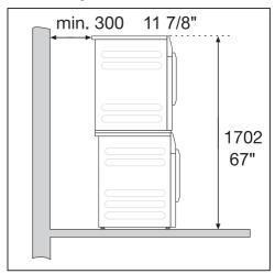
A stacking kit (APCL 001)\* is needed. This must be installed by a Miele authorized service technician.
