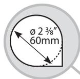
The  $\varnothing 2 \frac{3}{8}$ " (60 mm) services hole for the hoses should be enlarged to accommodate the extra venting hose by cutting out some material from the bottom corner.
