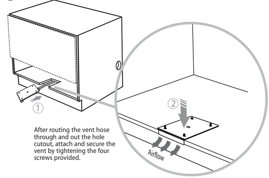
After routing the vent hose through and out the hole cutout, attach and secure the vent by tightening the four screws provided.
