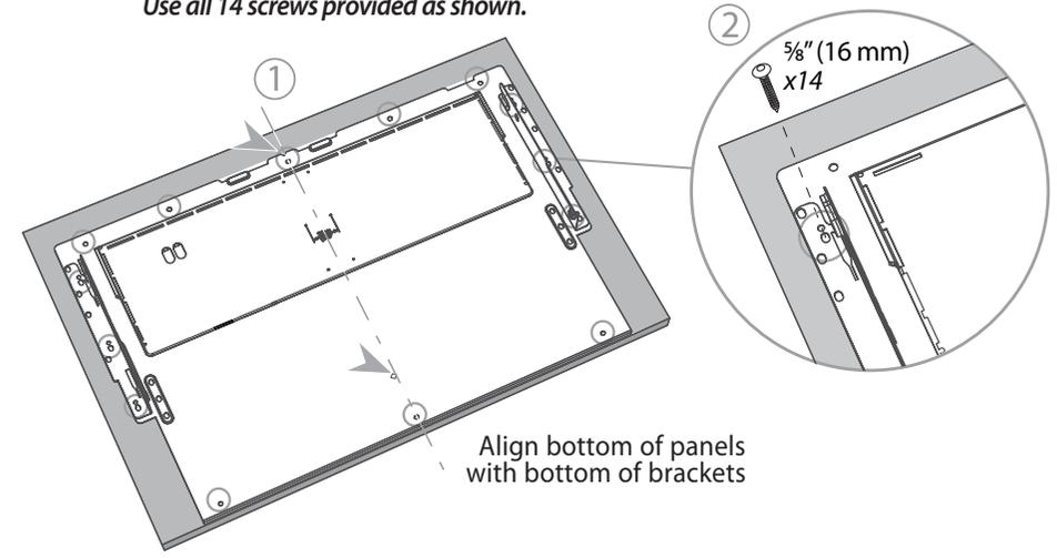
Align bottom of panels with bottom of brackets
