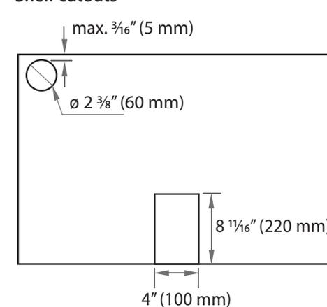
If the services holes are through metal, ensure you fit the supplied Edge Protector around the hole for the power cord.
