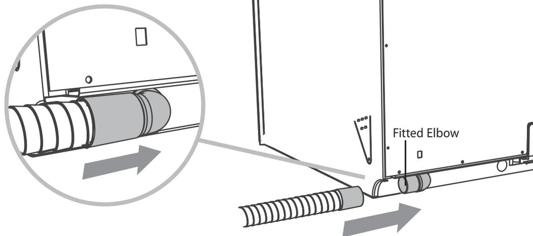
10b PULL THROUGH HOSES & MOVE INTO THE CAVITY
