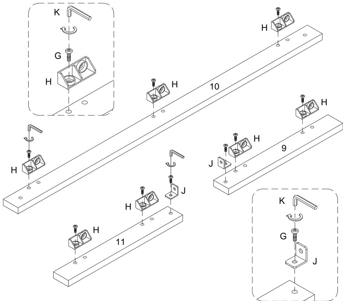
Using Bolt (G) attach plastic wedge (H) to parts (9,10,11) ,and using bolt (G) attach Connecting iron sheet (J) to parts (9,11) with Hex key (K) as per diagram.
