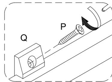
Using screw (P) secure plastic wedge (Q) with Philips head screwdriver as per diagram.
