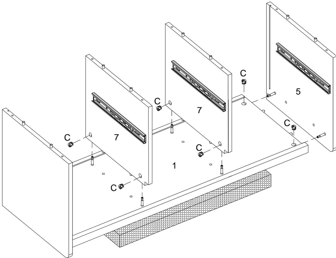
Using Cam lock(C) secure parts (5,7) to part (1) with Philips head screwdriver as per diagram.
