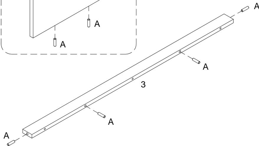
Insert wooden dowel (A) into parts (3,7) as per diagram.
