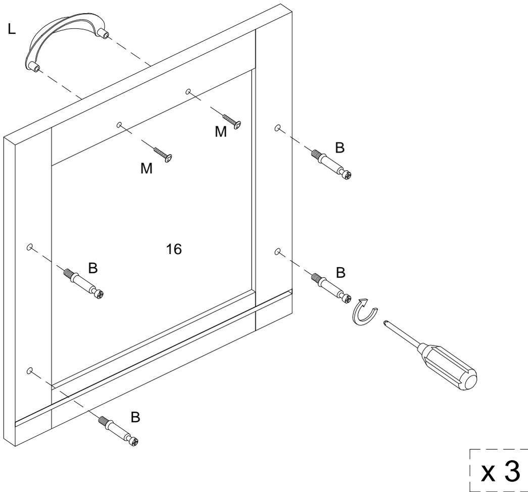
Secure cam bolt (B) into part (16), and using handle bolt (M) secure handle (L) to part (16) with Philips head screwdriver as per diagram.
