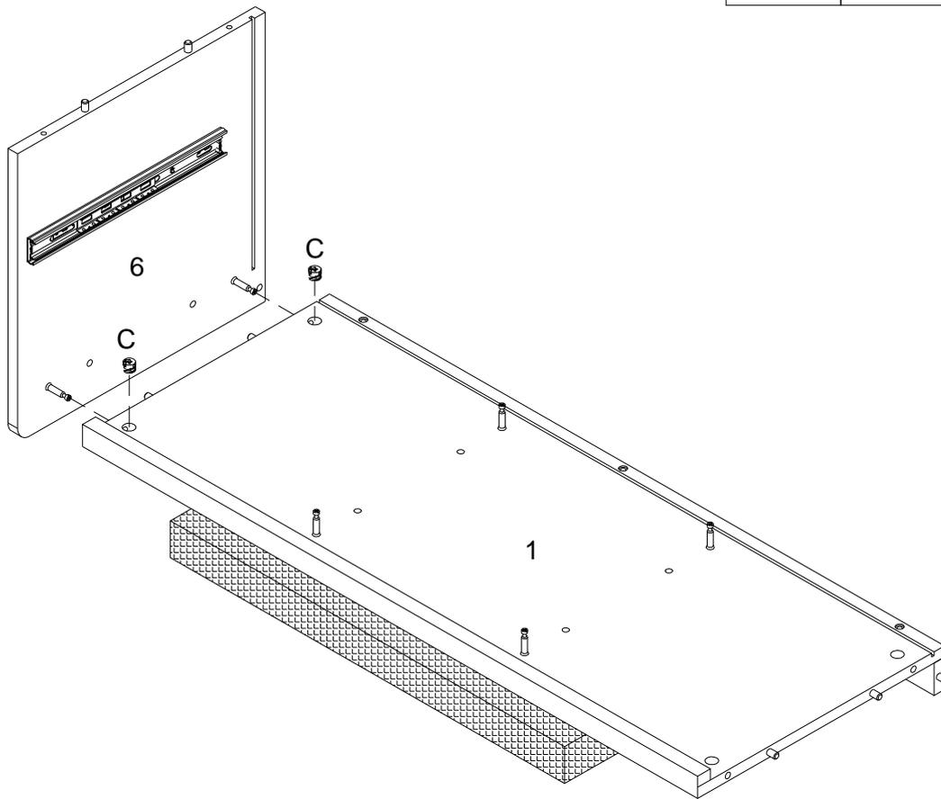
Using Cam lock(C) secure part (6) to part (1) with Philips head screwdriver as per diagram.
