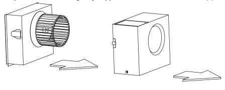
7) Remove the three screws retaining the blower motor(s). Unplug and remove the motor(s), taking care not to damage the blower wheel(s). It is not necessary to remove the blower wheel from the motor.
