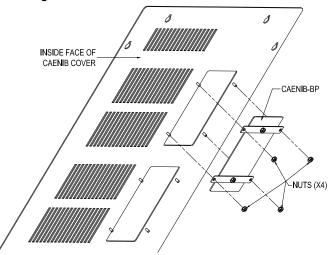
After positioning the blank plate to the CAENIB cover, use a wrench and the included nuts to secure the blank plate to the CAENIB cover. After all of the blank plates have been secured to the CAENIB cover, the cover can be installed on the CAENIB enclosure.
