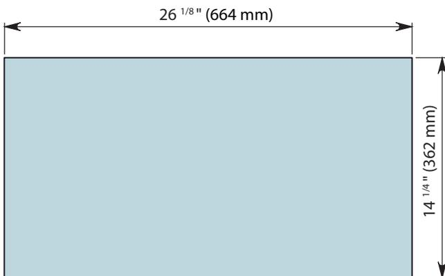
**EN - HOLE MEASUREMENTS FOR INSTALLATION**
