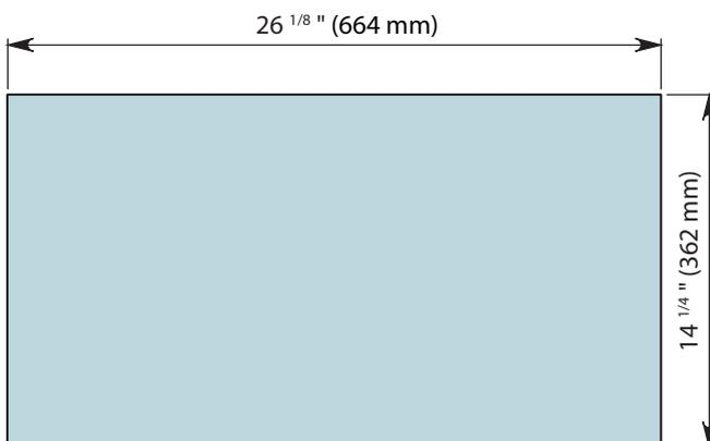
EN - HOLE MEASUREMENTS FOR INSTALLATION
