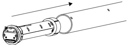
2. Ensure that a cusp on the motor crown aligns with the first screw hole in the roller tube. The cusp should be no further than 1/4 in (7 mm) off center of the screw hole. Ensure that the motor head is flush with the roller tube.
