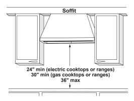
In this installation, the ductwork running from the top of the hood will be concealed in the soffit.
