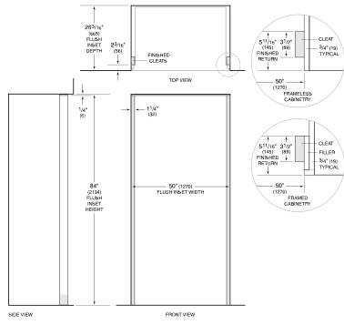
NOTE:  $3^{1}/2^{n}$  (89) finished returns and shaded areas will be visible and should be finished to match cabinetry. Shaded line represents profile of unit with  $^{3}/4^{n}$  (19) panel.
