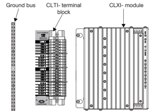
Terminal Block and Module Layout for a Double-Wide Enclosure (CLTI-2DIMU8 and CLXI-2DIMU8 Shown)
