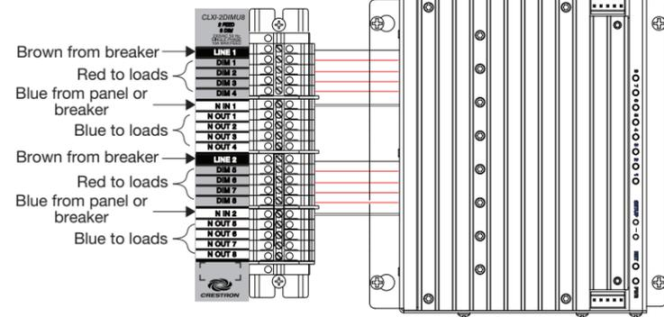
Removing the Line Jumpers after Testing (Single-Wide and Left-Side Double-Wide Enclosures and Right-Side Mounted CLTI-2DIMU8 Shown)
