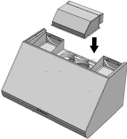
In the 30" version, it is possible to orient the air outlet towards the rear side of the cooker hood by rotating the sucking unit.
