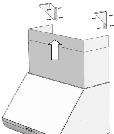
After having fixed the hood-bearing stirrup of the upper chimney, raise and block it with the two side screws.
