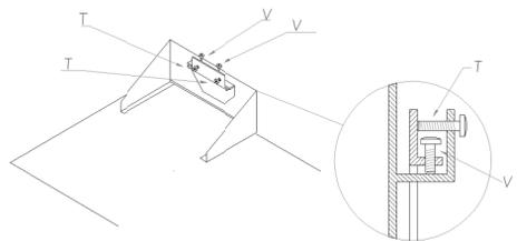
The air outlet of the product is oriented upwards: in the case that one prefers the air outlet towards the rear side of the appliance, it is only necessary to replace the air release piece with the other one supplied with the appliance.
