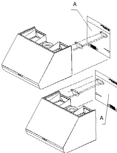
Hook the cooker hood into the bearings, then adjust vertically and horizontally the position of the appliance, acting on the special regulating metric screws.
