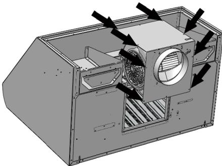
take the sucking unit out, rotate and reinsert it into the desired position, and then place again the screws that had been removed. To complete installation, insert the two fixing screws into the rear side of the cooker hood, into the two holes that were created beforehand. Before fixing the chimney in place, place the electrical feeding equipment into the decorative pipe as well as the related electrical connection.
