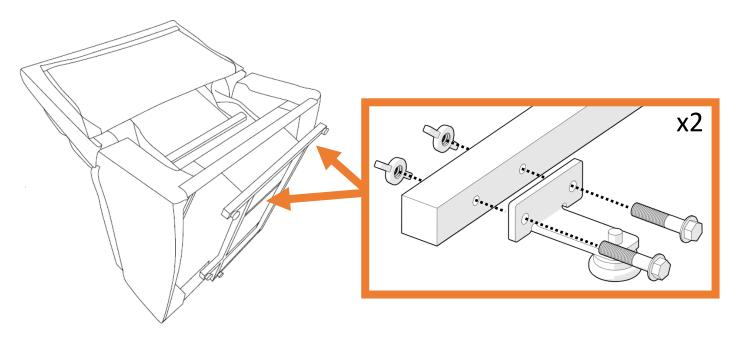
Adjust floor glides by twisting to ensure the base is level
