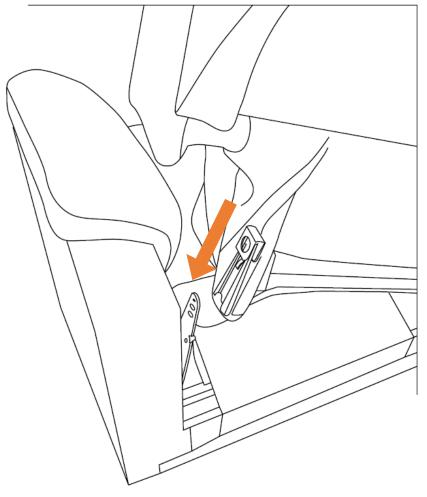
To install the back, align the female side on the back to the male side on the chair base and slide down until a click is heard.
