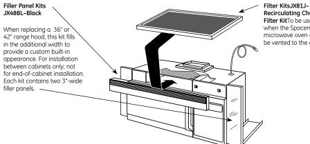
**Recirculating Charcoal** Filter KitTo be used when the Spacemaker microwave oven cannot be vented to the outside.
