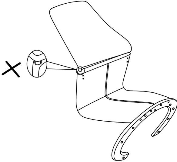
Step 2-a: Place the backrest (B) into the holes on the seat (A). Push down to make sure the screw holes on the backrest (B) are aligned with the screw holes on the seat (A). Screw in all necessary hardware as shown only halfway, do not completely tighten.
