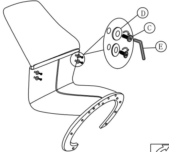
Step 2-b: Press the backrest (B) down so that the backrest is completely flush with the seat (A). Then proceed to completely lock all the screws. (Do not completely tighten the screws if the backrest (B) and seat (A) are not completely flush with each other)
