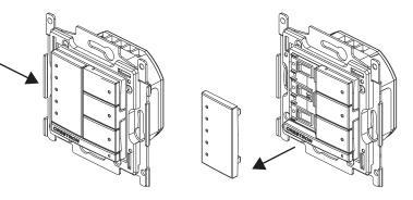
3. Insert the new button assemblies onto the device by pressing them into the device. It might be necessary to squeeze the sides of the button assembly to allow for easier assembly.
