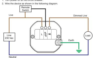
3. When making connections to the device, insert the wires into the back of the unit. Use a small flat head screwdriver to tighten the connection.
