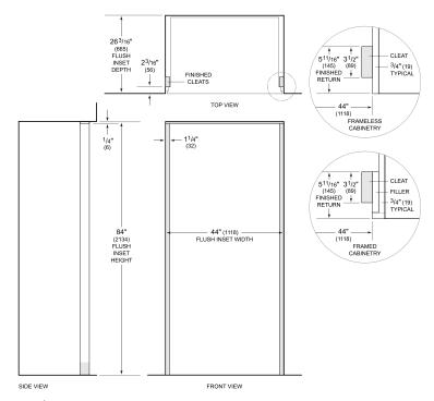
NOTE:  $3^{7}/2^{n}$  (89) finished returns and shaded areas will be visible and should be finished to match cabinetry. Shaded line represents profile of unit with  $3/4^{n}$  (19) panel.
