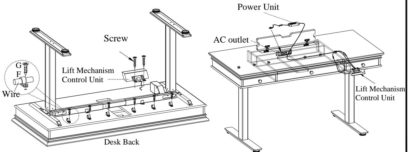
Note: Refer to Lift Mechanism assembly instructions for Control Unit operation.
