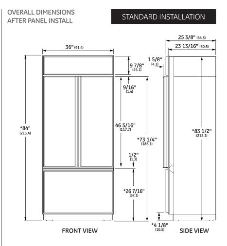
\*Shipping height. Use leveling legs and wheels for maximum 1" height adjustment from shipping height.
