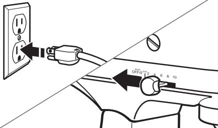
1 Plug the Stand Mixer into a grounded 3 prong outlet. Always set the speed control lever on lowest speed to start, then gradually increase speed to avoid splashing ingredients. See the "Speed control guide" to select the best speed for your recipe.
