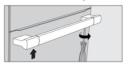
■ Tighten the four screws with the screwdriver supplied.
