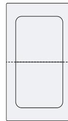
If the function is active on one cooking zone segment and you set a power level on the other cooking zone segment, the function will be deactivated. The cooking zone is automatically set to power level 9.
