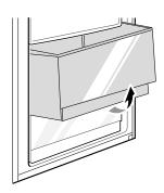
2 To reassemble, slightly tilt up the front, insert the crisper into the frame and push it back into place.
