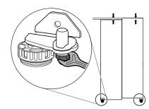
Open the door and use the wrench 10 to loosen the keeper nut by turning it to the left.
