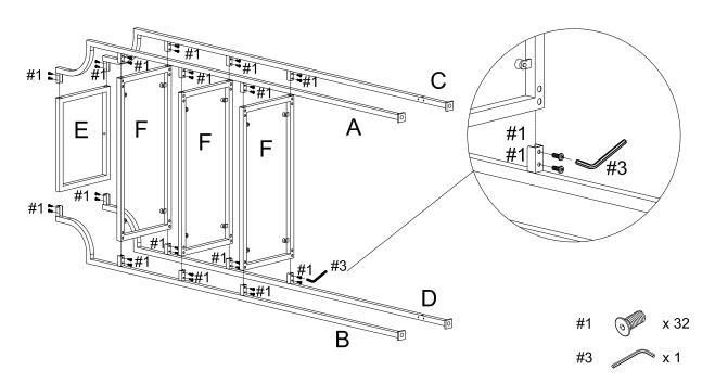
Step 2. Carefully turn unit upright. Attach cross bars (part H) between front legs and back legs (parts A & C, B & D) using sunk bolts (part #1) and allen wrench (part #3).
