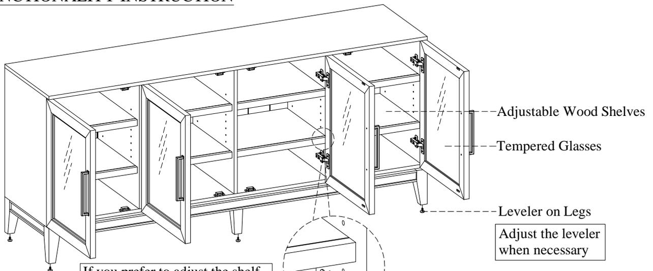
If you prefer to adjust the shelf location, remove the screws and move shelf brackets to the desired location. Then secure the brackets to shelf with screws.
