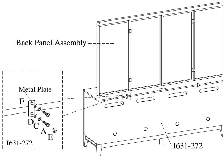
**STEP 4:** Attach the side assemblies to the console/back panel assembly by using 8 bolts(A), lock washers(C), flat washers(D) with 4 metal plates(F) as shown below. Do not completely tighten bolts.
