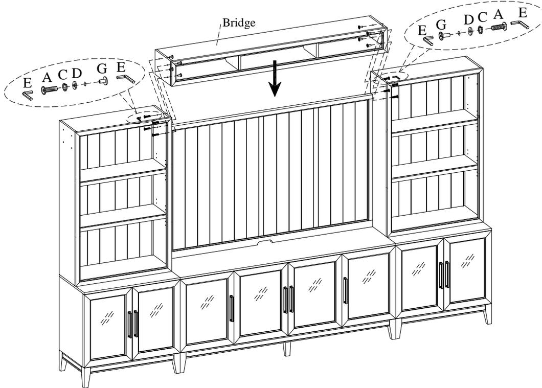
**STEP 6:** When the combination is complete, insert plastic plugs("F" on the hardware bag of the pier hutch) into the holes on both side panels as shown below.
