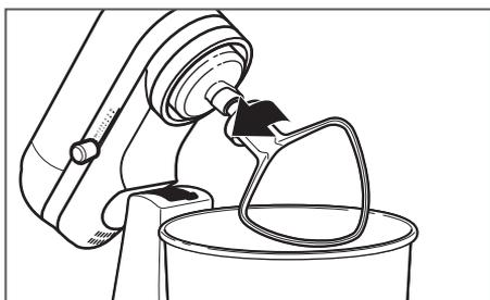
**2** **Remove the accessory:** Turn the speed control to "0", unplug the Stand Mixer, and tilt the motor head back; then, press the accessory upward as far as possible, turn the accessory clockwise and pull it away from the beater shaft.
