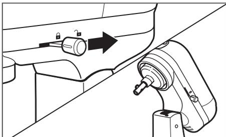
**1** **Raise the motor head:** Check to be sure that the Stand Mixer is unplugged, and the speed control is turned to "0"; then slide the locking lever to the unlock position and lift the motor head. Once lifted, slide the locking lever to the lock position to keep the motor head up.
