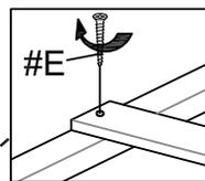
2. Align the ends of the slats (#6) to the side rails (#5), then insert a screw (#E) into each end and secure using the a Phillips screwdriver.
