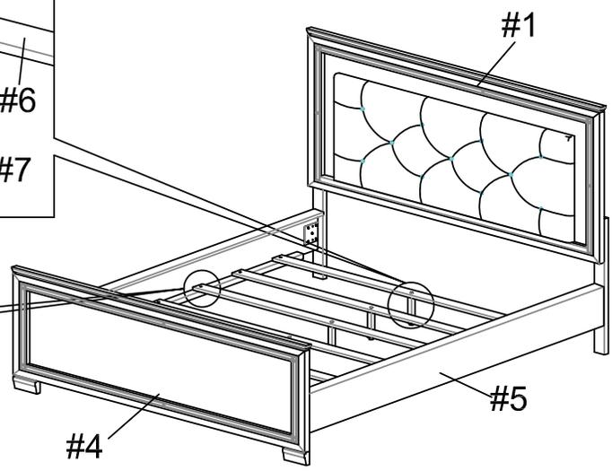
2. Align the ends of the slats (#6) to the side rails (#5), then insert a screw (#E) into each end and secure using the a Phillips screwdriver.
