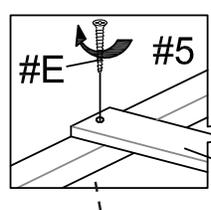
2. Align the ends of the slats (#6) to the side rails (#5), then insert a screw (#E) into each end and secure using the a Phillips screwdriver.
