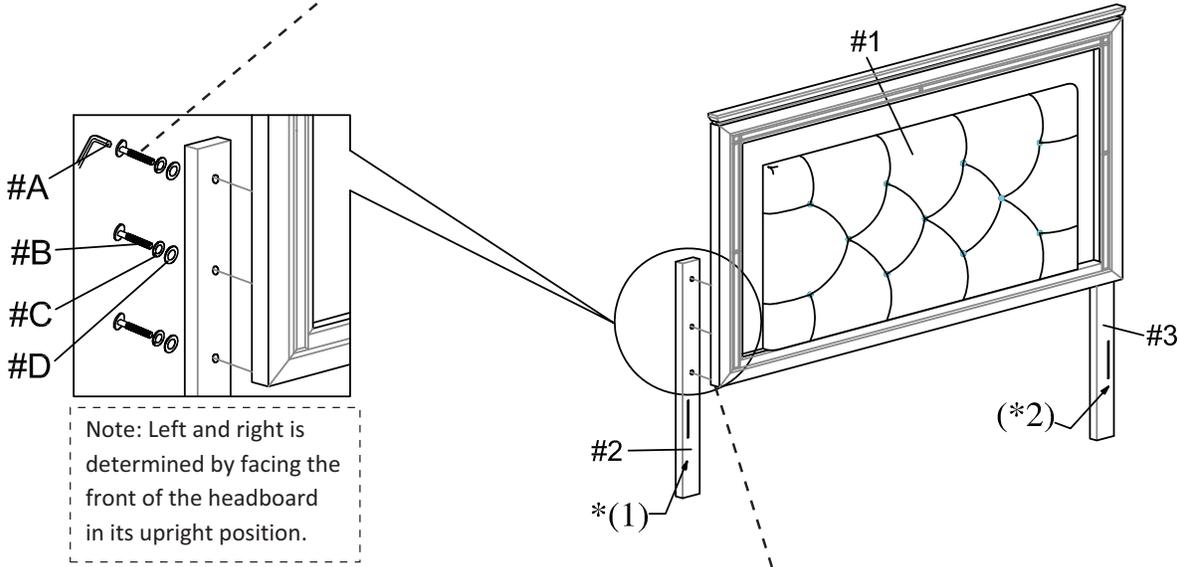
2. Align the right and left headboard legs (#2,3) to the holes along the sides of the headboard (#1), then insert 3 bolt assemblies into each leg and secure using the Allen wrench (#A).
