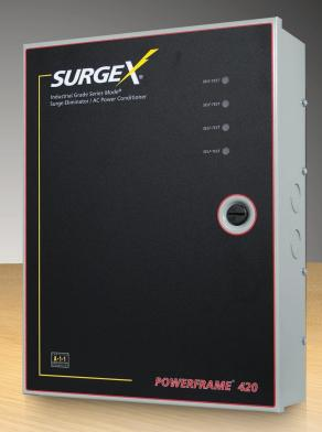
The PF-420 is the perfect protection solution for multi-circuit residential AV systems where space is at a premium. This compact 120 Volt / 80 Amp load center is hardwired as a subpanel at the service panel or the equipment room and is designed to provide robust protection required for multi-branch circuit applications.
