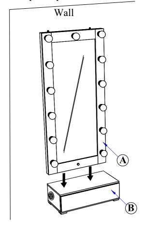
STEP 3: Please align and touch tall mirror(A) at the wall. Please marking and drill hole for Insert Wall plug(2) to the wall. Then secure Tall Mirror (A)with flat head chipboard screw(1) and tighten with screw driver(not included )as shown.
