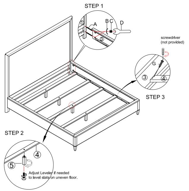
Step 1: Attach Rails (3) to Headboard (1) and Footboard (2) by using Threaded Rods (A), Curved Washers (B) and Nuts (C), tighten them with Open Wrench (D).
