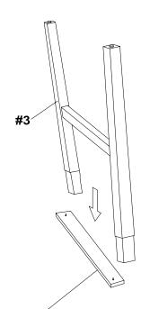
Remove the shipping cleat from end of front leg assembly #3.
