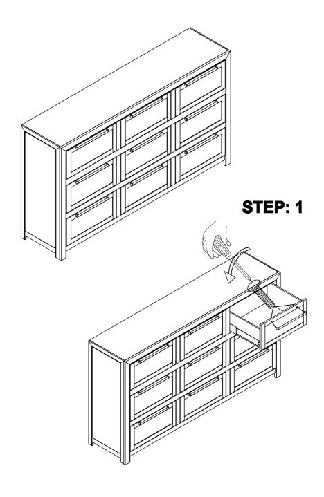
Open the drawers, unscrew the handle(s) from inside, install it on the outside, and tighten the screws.
