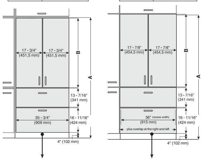
The height of this panel cannot be reduced for higher toe kicks as it will reveal structural elements of the appliance. Instead, install appliance on a platform and adjust the opening height to accommodate.
