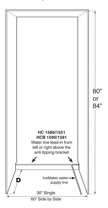
Concerning the refrigerator compartment there is the option to choose between stainless steel panels for a 80" or a 84" installation situation.
