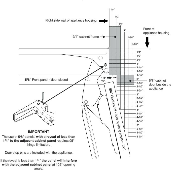
When the hinge is limited to 95°, the minimum reveal is 1/8".
