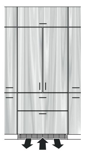
It is important to use the provided cover grille for the ventilation opening. This opening must not be covered.
