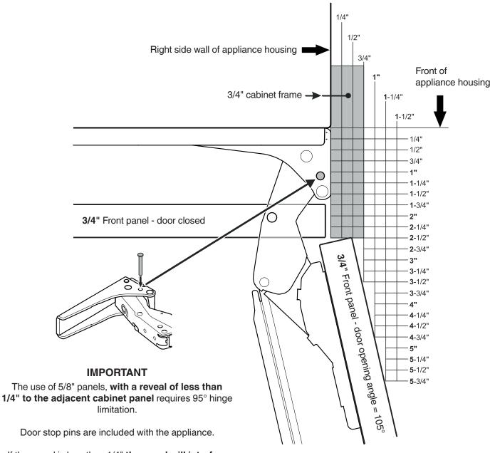
If the reveal is less than 1/4" the panel will interfere with the adjacent cabinet panel at 105° opening angle.
