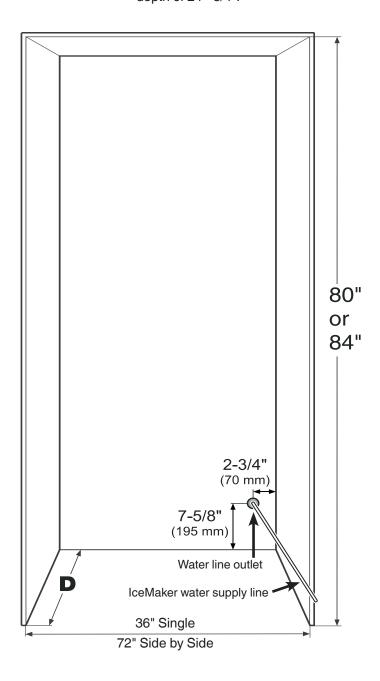
Concerning the refrigerator compartment there is the option to choose between stainless steel panels for a 80" or a 84" installation situation.
