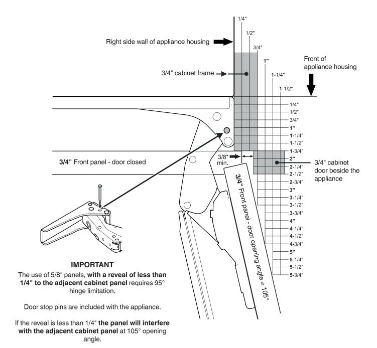
When the hinge is limited to 95°, the minimum reveal is 1/8".
