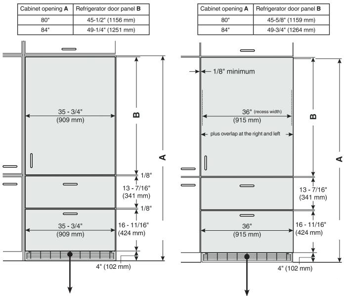
The height of this panel cannot be reduced for higher toe kicks as it will reveal structural elements of the appliance. Instead, install appliance on a platform and adjust the opening height to accommodate.
