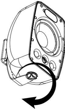
7. Connect the wire to the amplifier, and make sure the wire is correctly routed: eg: the left speaker output will be routed to the left speaker, right output to right speaker, etc. To connect the wire from the amplifier to the phoenix connector on the front speaker baffle:
