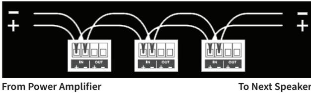
**7d.** Determine the proper wattage setting for each speaker in the installation and set each speaker's Transformer Tap selector on the front of the speaker accordingly. eg: You can set the tap to 70V Wattage or 8 ohm. Then fit the wiring terminal cover in the speaker front panel.
