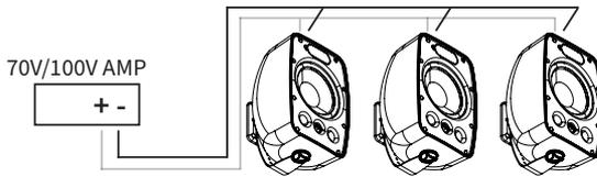
Wiring Diagram for 8 Ω system
