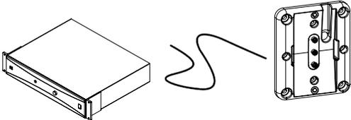
2. Attach the mount bracket to the mounting surface using 4 screws (not included), using studs or anchors, that are appropriate for the type of surface.
