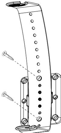
6. Attach the speaker to the C-Bracket, using the screw down caps and adjust correct horizontal angle.
