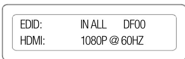
To change the EDID value for source inputs using the Matrix front panel buttons press the following:-
