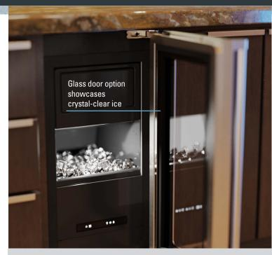
Much like a fine chocolatier slowly tempers chocolate to a solid state for the best quality and flavor, Marvel Clear Ice employs a fractional freezing process to create clear ice with the ultimate clarity and purity. As water runs over the cold plate, pure water freezes first. Dissolved solids are carried away into the water reservoir, giving you clear ice that cools your drinks without affecting the flavor.
