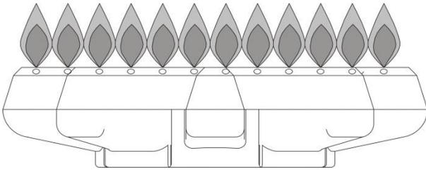
A properly adjusted burner will have sharp conical shaped blue flames. However, on some larger burners (22,000 BTU or 25,000 BTU) the cones are close together and blend into one another. The flame should be almost all blue. If your flames do not appear, follow the instructions to adjust the air shutter.
