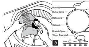
Turn the cycle knob to Water Faucet and press and hold the Start Button to turn on, press the Pause button or Power button to turn off.
