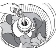
**NOTE:** When using fabric softener, always use the Soil & Rinse knob to select a setting with '+Extra Rinse.' This will ensure that no fabric softener remains on clothing after the cycle is finished.
