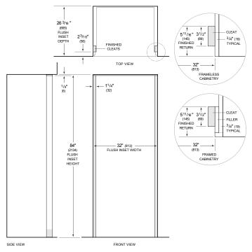
NOTE: 31/2" (89) finished returns and shaded areas will be visible and should be finished to match cabinetry Shaded line represents profile of unit **b**it (19) panel.
