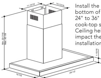
Install the hood so the bottom of the hood is 24" to 36" above the cook-top surface. Ceiling heights may impact the final installation distance.
