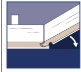
Step 2: Lock short end of flooring by inserting tongue into groove at an into groove at an angle and drop in place. At end of the row, measure and cut the flooring to complete the row. Install the cut edge closest to the wall.
