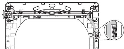
**6** Remove 2 screws and top lock rod holder. Set the lock rod holder and screw aside.
