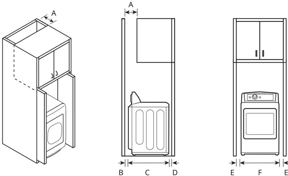
For cabinet installation with a door, minimum ventilation openings in the top of the cabinet are required.
