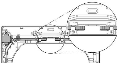
**10** Reverse the **9** lower hinge bracket and **11** hinge assembly.
