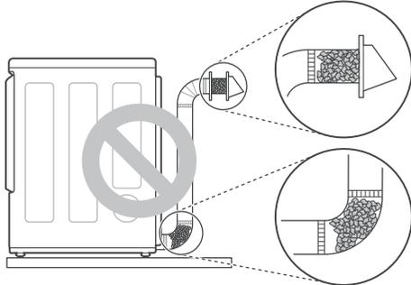
**Make sure the ductwork is not crushed or restricted.**
