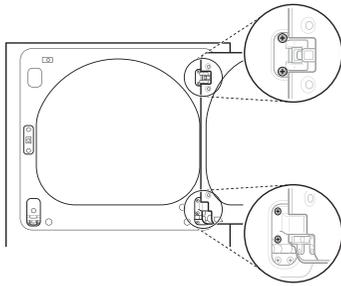
**2** Remove the four hinge screws.
