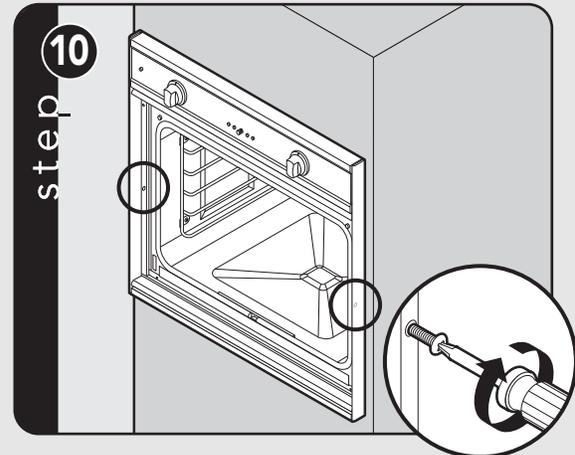
Attach screws to the side of the framing.
