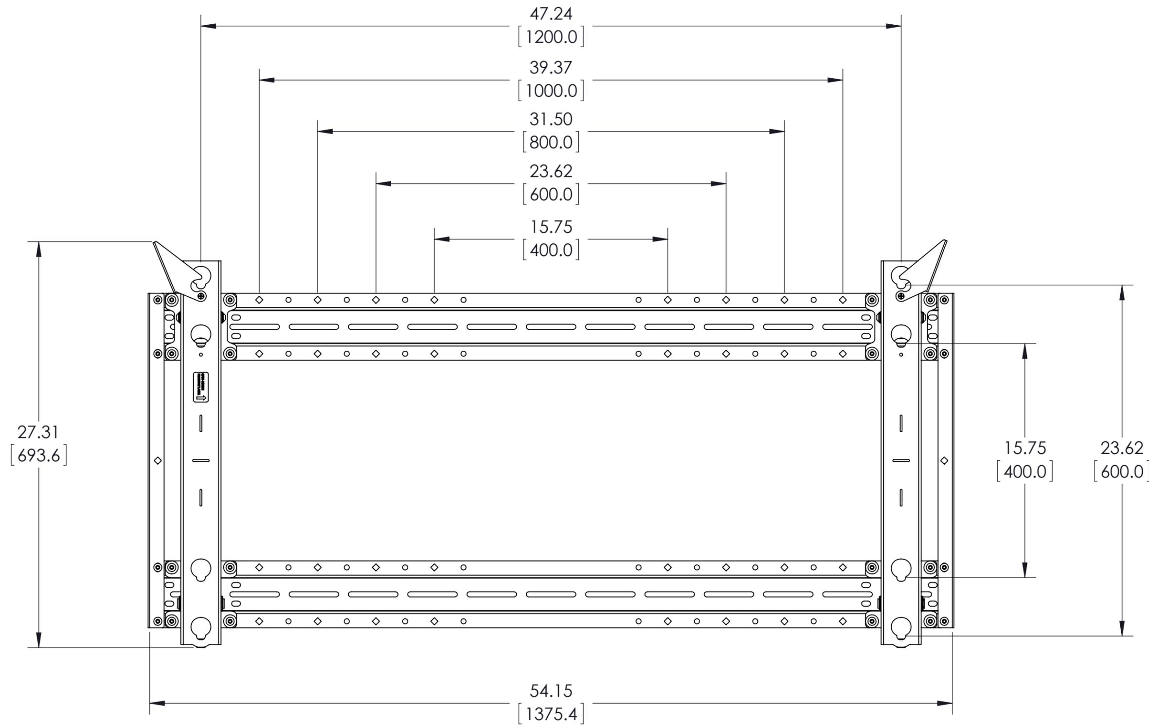
**SHOWN SET UP FOR A SCREEN WITH A MOUNTING PATTERN OF 1200 mm WIDE X 600 mm TALL**
