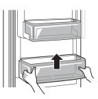
**2** To assemble the bin, slide it in above the desired support and push down until it snaps into place.
