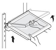
**2** Pinch the sides to open the water filter cover.
