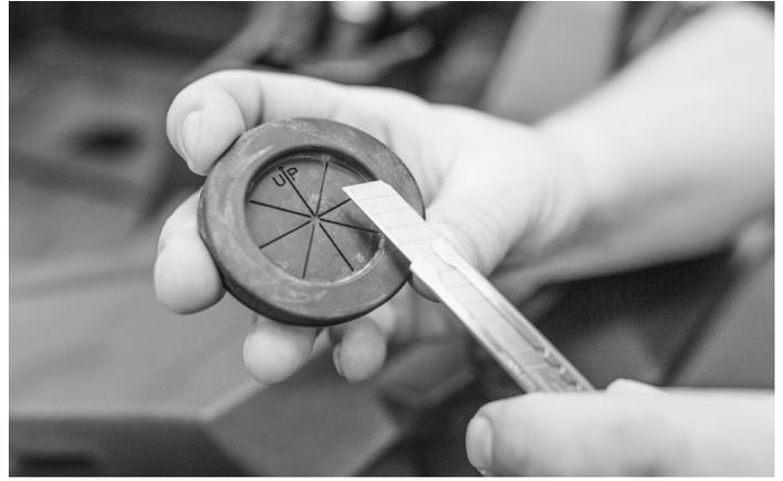
Remove the existing rubber grommet in the fire wall and cut along the score lines to open it up for the wire harness.
