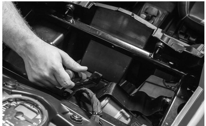
Be sure to slide the pocket support onto the rear brace for a secure fit.
