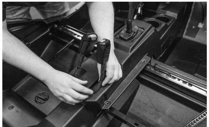
Disconnect the rubber boots on the shifter and seat belts by squeezing them inward to loosen them from the console.
